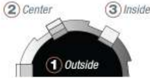
TRI-CUT SYSTEM There are three different edged cutting blades. One blade slanted outward, one toward and one that peaks in the center. This arrangement balances the cutting effort for smooth boring, better control and less chance of excess drag.
