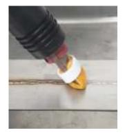
The SURFOX electrochemical cleaning process uses the power of electrical current and the electrolyte cleaning solution to remove heat tint without altering or damaging the surface of the material. It will leave a clean surface, free of residue and promote the formation of a uniform and durable chromium oxide passive layer to protect stainless steel against further oxidation.
